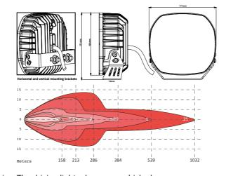
A trendsetter in the LED driving light range: the TRALERT® Phantom Series. The driving light when your vehicle deserves or requires only the best in optics and functionality. The Phantom Series 7" is available with a black housing (Art. WD-13013). Despite its smaller size, this driving light has a light output of no less than 12,000 lumens, resulting in excellent visibility in all conditions.
