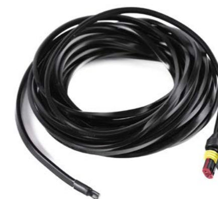
Verlengkabel 800cm 1x 0,75mm 2 - 1x 2-PIN Superseal (Art. KAC-80005S)
