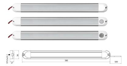
The B-2038 series interior lighting is the shortest variant of the B-2000 series interior LED strips. These strips are 380mm long and deliver a light output of 750 lumens. With a light colour of 6500K, this lamp delivers neutral light similar to natural daylight. This bright colour increases concentration and performance in the room making this very suitable for the interior of your commercial vehicle.
