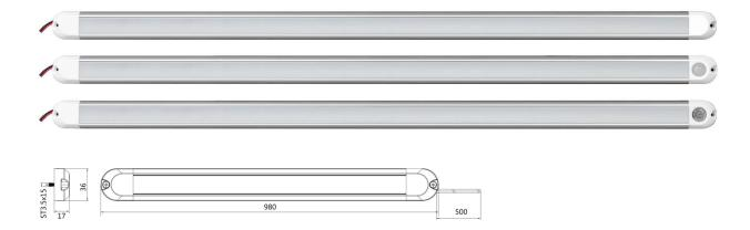
The B-2098 series interior lighting is the longest variant of the B-2000 series interior LED strips. These strips are 980mm long and deliver a light output of 2250 lumens. With a light colour of 6500K, this lamp delivers neutral light similar to natural daylight. This bright colour increases concentration and performance in the room making this very suitable for the interior of your commercial vehicle.
